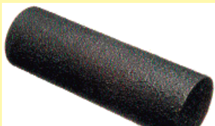
Figure 1a: Cast iron specimen from the outer side of the side wall.
