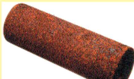
Figure 1b: Cast iron specimen from the inner side – showing corrosive attack.
