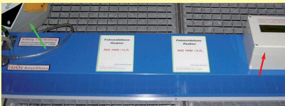
Photo-oxidation and sterilization reactor (green arrow: addition of hydrogen peroxide, red arrow: electronic control).
